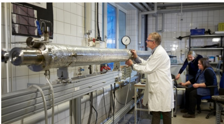
Photo: Staffan Nyström, Gunilla Pettersson and Birgitta Engberg works in the laboratory with dynamic material testing – using the encapsulated split-Hopkinson pressure bar device.
