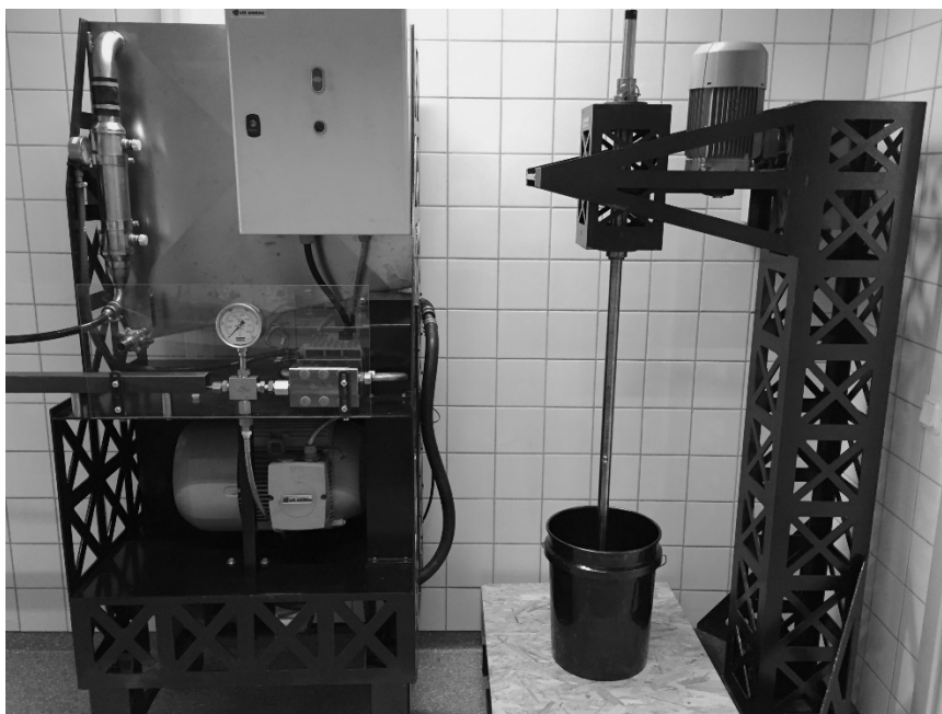
Figure 1: The hydrodynamic tube shear system (left) and its cooperating stirrer (right).
