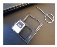
Check out what size it is on the current sim-card and how it is placed. Remove the new sim-card with the right size and place it in the slot where the old sim-card was.
